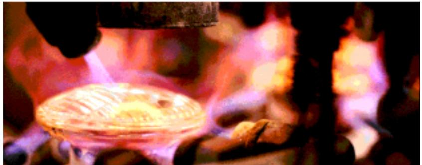
**Glass lamp lens being heated during the 'fuse seal' process. This work is performed by members of Local 1627, Lexington, Kentucky.**
